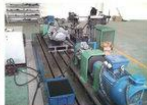
汽车手动变速箱同步器性能测试平台 Automobile Manual Gearbox Synchronizer Performance Test Platform
